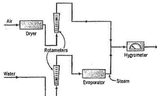
Steam and dry air are fed at known flow rates and mixed to form a gas stream with a known water content, and the hygrometer reading is recorded; the flow rate of either the water or the air is changed to produce a stream with a different water content and the new reading is recorded, and so on. The following data are taken:
